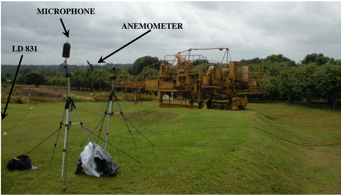
Equipment Setup C: Larson Davis 831 Sound Level Meter with Weather Module
